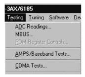
Both 1900MHz and 800MHz CDMA is started from the same selection of "Testing" and "CDMA". Entering this screen switches on both the transmitter and receiver on Channel 364. For PCS simply click the PCS box. The PDMs can be adjusted with the slider or by entering a value. The transmitter is switched off by clicking the "Tx Off" Box. The RX\_IF\_AGC is read by clicking the "Read" button. The LNA defaults to ON and OFF can be switch by ticking the "LNA" box.
