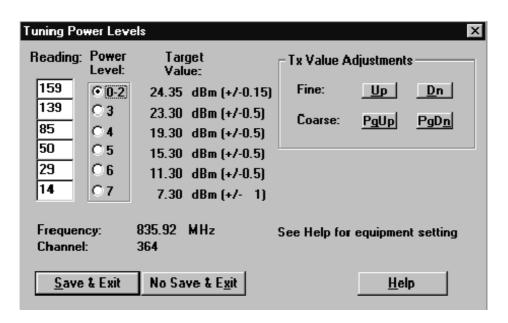
**NOTE:** This window was taken from WinTesla with the cable loss set at 0.7dB. The power levels tuned at the phones RF connector are:
