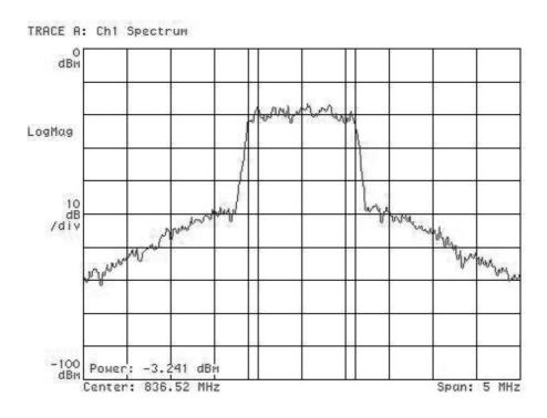
Tx Output spectrum at RF Connector with 30dB attenuator on Spectrum Analyzer:
