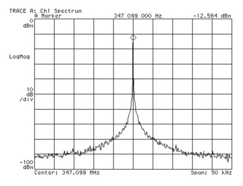
UHF Cel LO measured at Odyssey N703 Pin 2 (TP106) with Hi Z probe when set to Channel 384:
